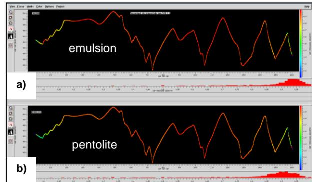
Fig. 5. Elevation vs. line distance, with color indicating the percentage of traces per shot with geological response larger than noise. In (a) the emulsion and in (b) the pentolite shot lines. Color scale: blue 0%; green 50%; red 100%. Below each plot is the histogram of the percentage (0-100%).
