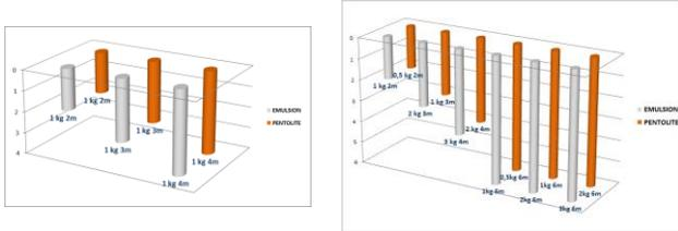
Fig.1. Explosive charge and hole depth for the 18 shotpoints of first (left) and second (right) steps. Grey is for emulsion and orange for pentolite.
