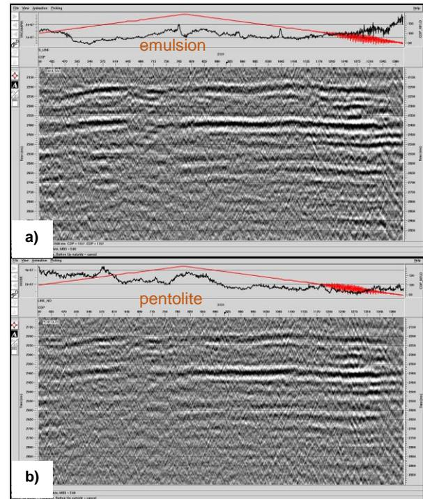
Fig. 3. Zoom of the seismic sections for the emulsion (a) and pentolite (b) lines. The pentolite/emulsion charge is 2kg/3kg per shot. Vertical axis: time (2100ms to 3000ms). The Red curve stands for the *cdp* fold (scale from 50 to 200). The black curve stands for noise *rms* amplitude. In (a) the scale is from  $0.5 \times 10^{-7}$  to  $3 \times 10^{-7}$  V. In (b) it is from  $0.5 \times 10^{-7}$  to  $6 \times 10^{-7}$  V.
