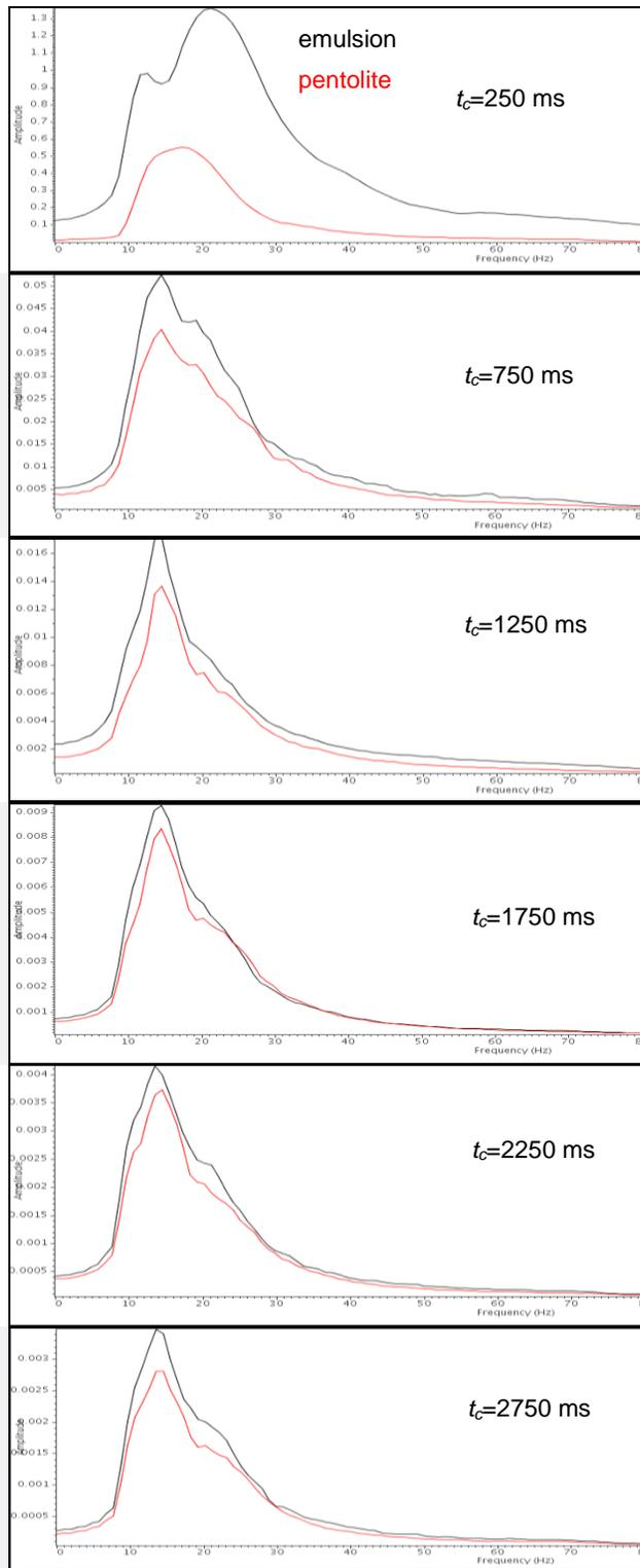
Fig. 4. Amplitude spectra from a time window of 500 ms centered at  $t_c$  along the seismic section of the emulsion (black) and pentolite (red) lines.
