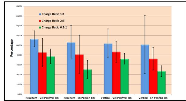
Fig.2. Percentage of pentolite/emulsion ratio of both resultant and vertical velocities and energies for charge ratio of 1:1 (blue); 2:3 (red); and 0.5:1 (green). On top of each bar is the center of the error bar.
